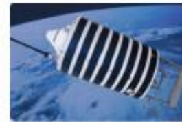
The first Russian nanosatellite TNS-0 №1 (launched in 2005), passive magnetic attitude control system, 4.5 kg (credit JSC "Russian Space Systems" )
