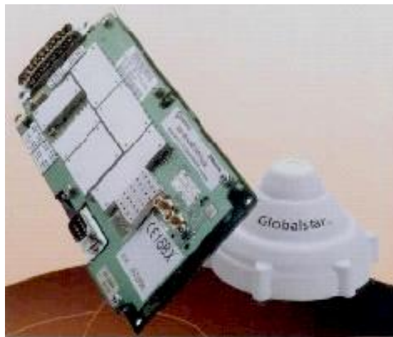
Fig.6. The GLOBALSTAR satellite communication unit (modem and antenna)
