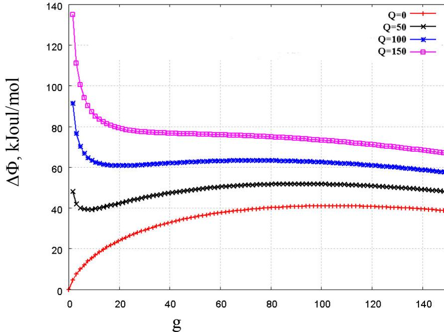
**Fig.2** Dependence of the thermodynamic potential of the nucleus formation for melted spherical drops in plasma discharge from drop size  $g$  for several charges of drops is presented.  $g$  is size of cluster,  $g$  is measured in number of *Si* and *C* atoms in cluster.  $Q$  is drop charge.  $Q$  is measured in  $1.6 \cdot 10^{-16}$  coulomb.
