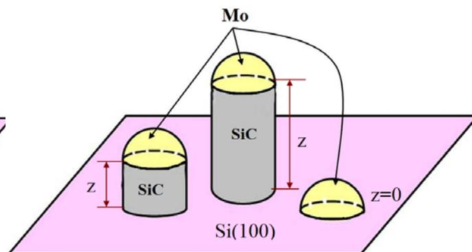
**Fig. 20** Scheme of  $SiC$  nanowhiskars formation under irradiation of gas mix contained carbon is presented.
