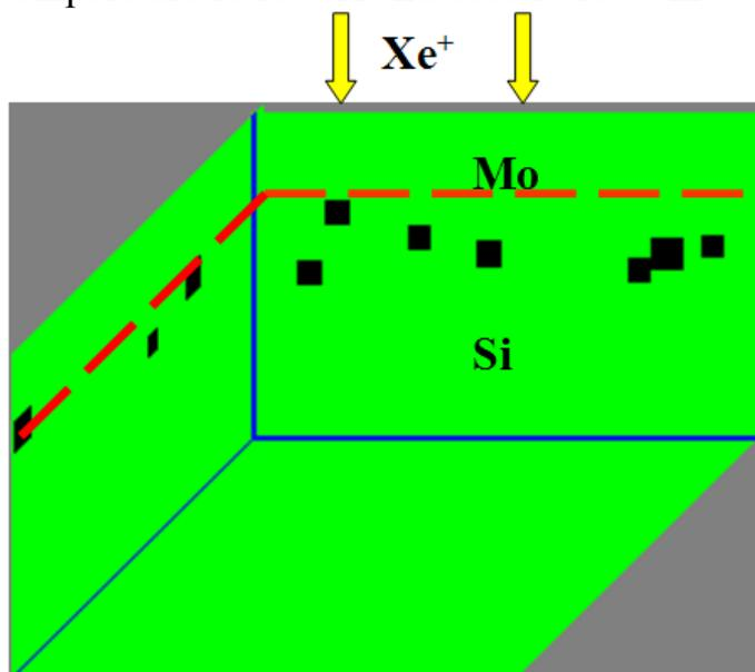
**Fig. 12.** Illustration of blisters formation in the bilayer substrate consisting of layer *Mo* and layer of crystal *Si* is presented. *Mo* width is 94 Å, *Si* width is 543 Å. Black color corresponds porosity, and green color lack of porosity in this point. Temperature is 1000K,  $Xe^{++}$  ions energy is 5keV, irradiation dose is  $10^{15}$   $cm^{-2}$ . Long-size defects structures don't format.
