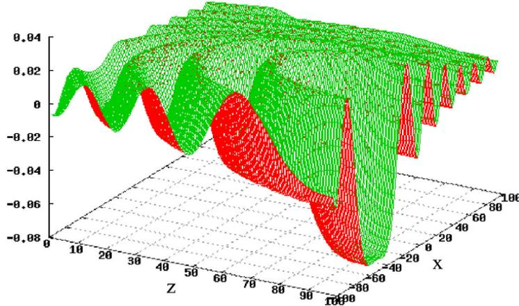
**Fig. 5.** 2D projection of equal potential (blister-blisters) values as surface  $U(x, y=\text{const}, z)$  is presented for  $y=0$ . The value of potential is presented in dimensionless units.  $X$  and  $z$  is measured in lattice parameters of *Si*.
