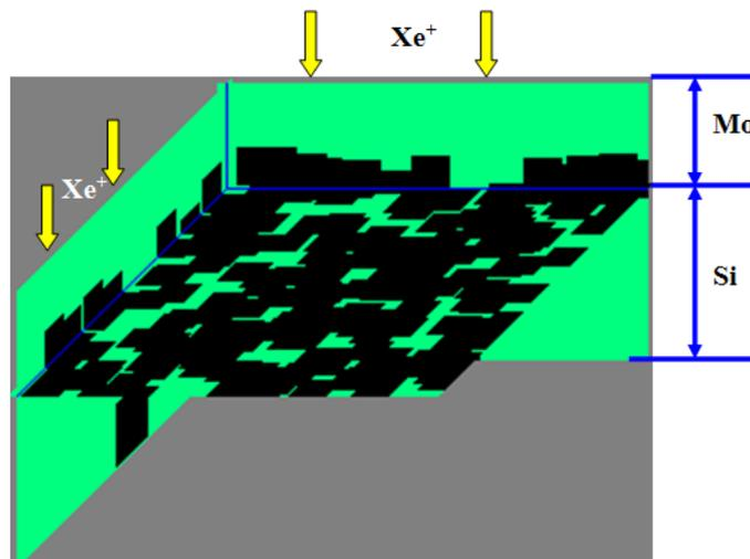
**Fig. 18** Illustration of long-size structures of defects on  $Mo/Si$  surface are presented.
