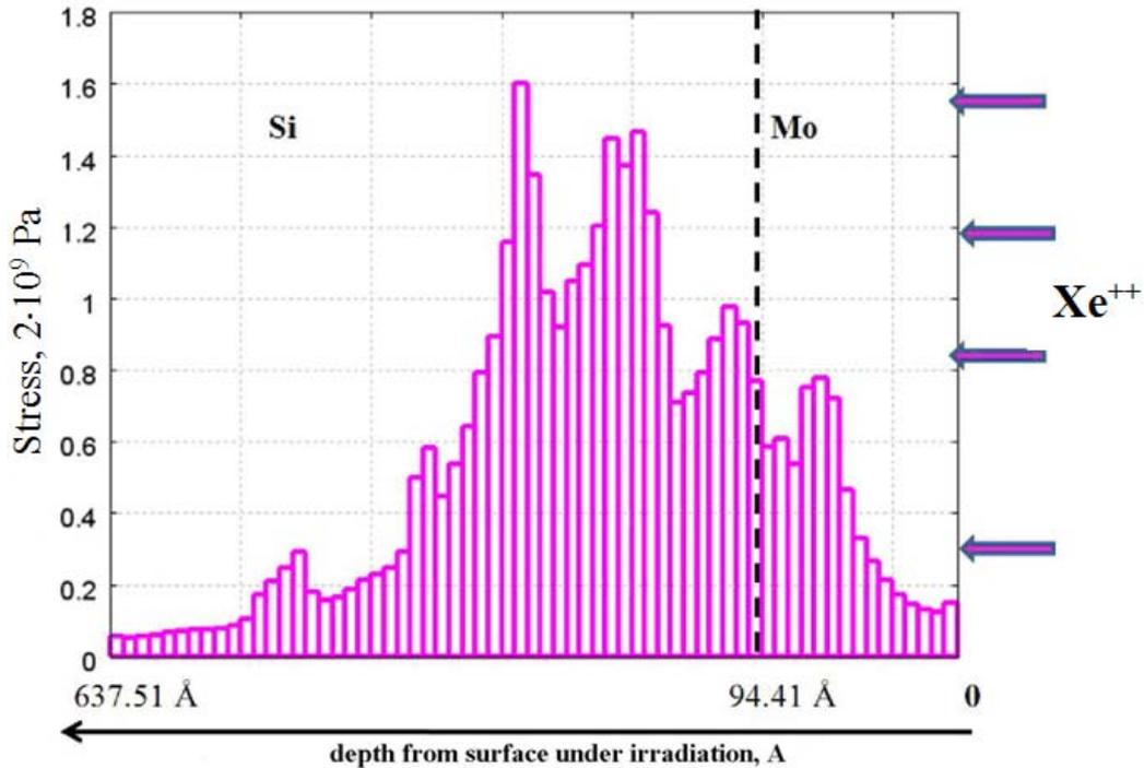
**Fig. 7.** Stress in layers of substrate averaged for x and y coordinates is presented.
