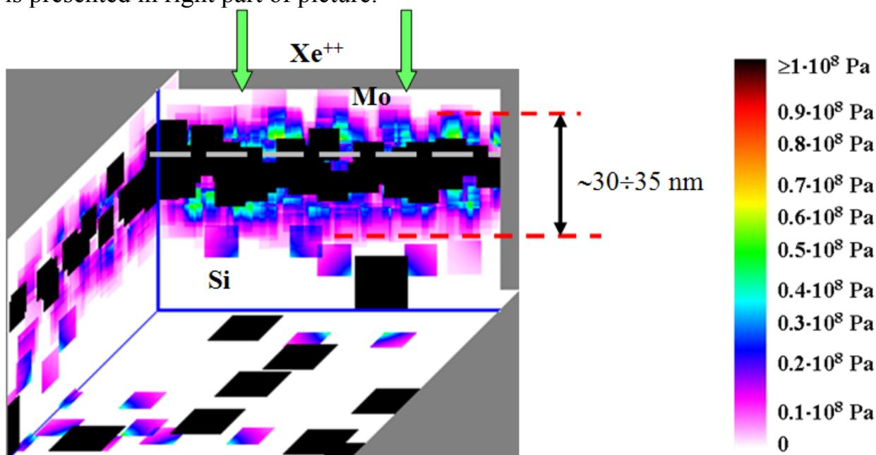
**Fig. 16** Stress corresponding with blistering in some section of substrate is presented at finish of fluctuation stage ( $10^{-4}$ s). Temperature is 1000K,  $Xe^{++}$  ions energy is 5keV, irradiation dose is  $10^{16}$   $cm^{-2}$ . Palette of correspondence of stress value and color is presented in right part of picture.
