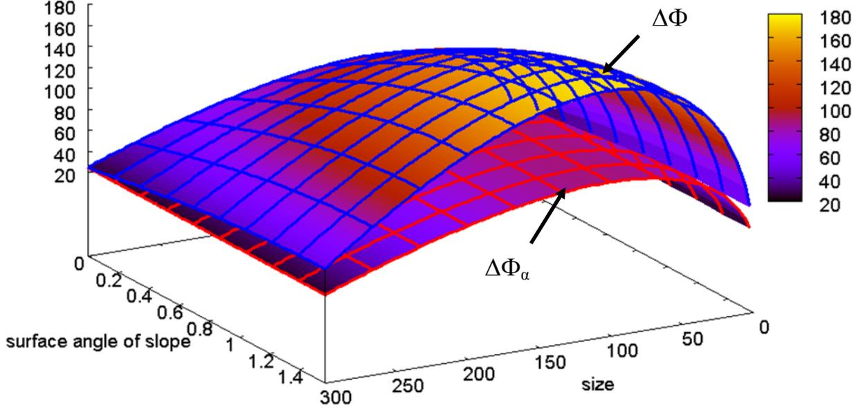
**Fig. 4** Comparison of Gibbs energy for *SiC* formation on sloping surface ( $\Delta\Phi_\alpha$ ) and Gibbs energy for *SiC* formation on surface without slope ( $\Delta\Phi$ ) is presented for inclination of plane from 0 to  $\pi/2$ .
