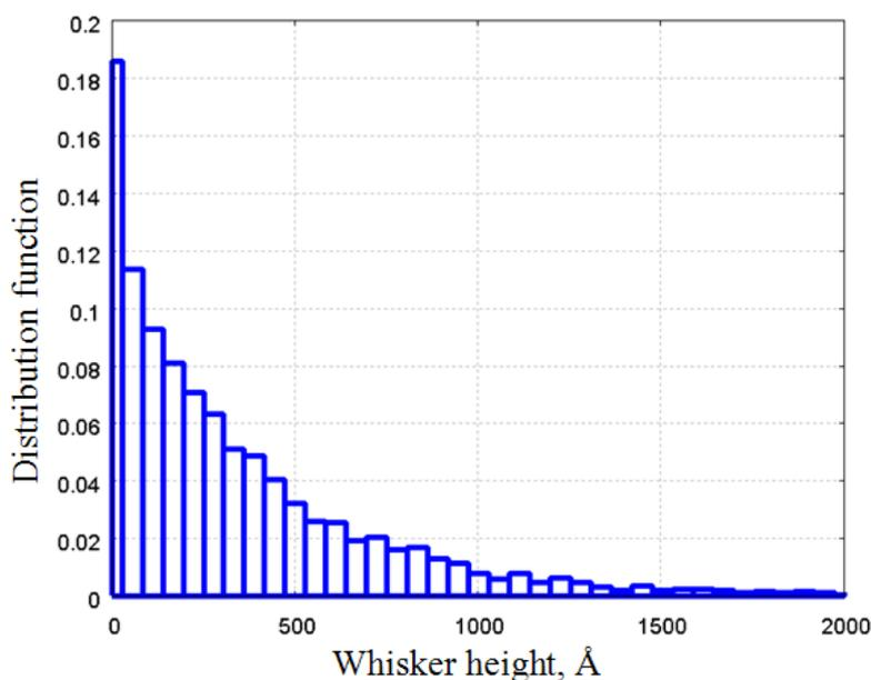
**Fig. 21** Distribution function of  $SiC$  whiskers on  $Si(100)$  with  $Mo$  catalysts is presented at finish time of calculation. Radius catalyst is  $\approx 9,8\text{\AA}$  ( $\approx 3$   $Mo$  lattice parameters), catalyst density is  $3,39 \cdot 10^{12} \text{ cm}^{-2}$ , substrate temperature is 900 K.  $10^6$  trajectories are used.
