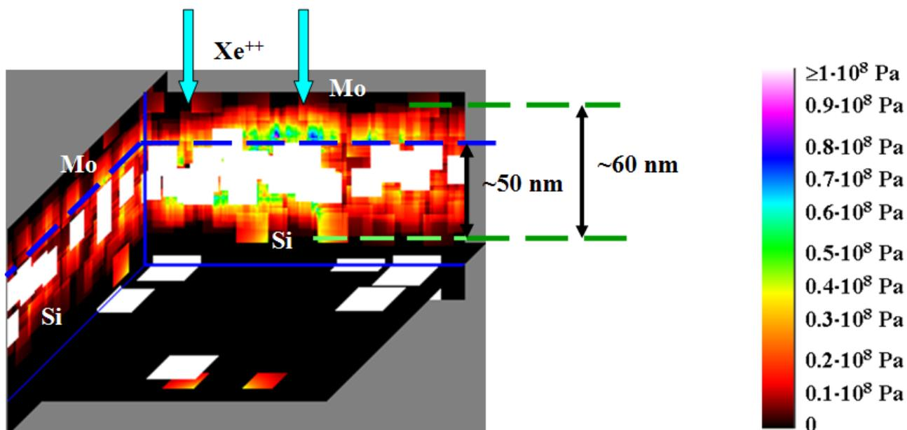
**Fig. 15** Stress corresponding with blistering in some section of substrate is presented at finish of fluctuation stage ( $10^{-4}$ s). Temperature is 900K,  $Xe^{++}$  ions energy is 5keV, irradiation dose is  $10^{16}$   $cm^{-2}$ . Palette of correspondence of stress value and color is presented in right part of picture.
