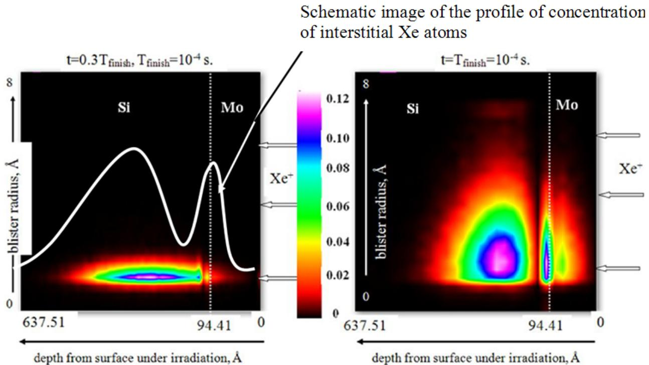
**Fig. 6.** Color visualization of blisters DF averaged for the  $x$  and  $y$  coordinates from blister size and its depth from surface under irradiation is presented at two time moments: 0.3 duration of fluctuation stage and at finish of calculation.
