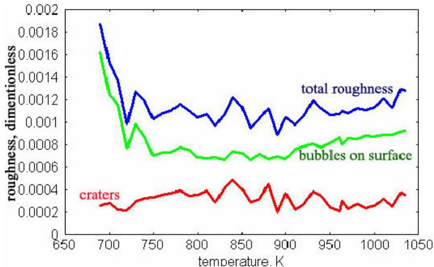
**Fig. 22** The roughness (dimensionless ordinate) versus design temperatures (abscissa) is presented.
