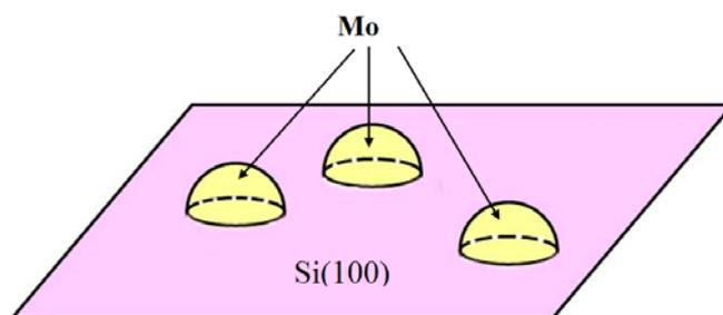
**Fig. 19** Scheme of  $Si(100)$  surface after  $Mo$  layer peeling is presented.
