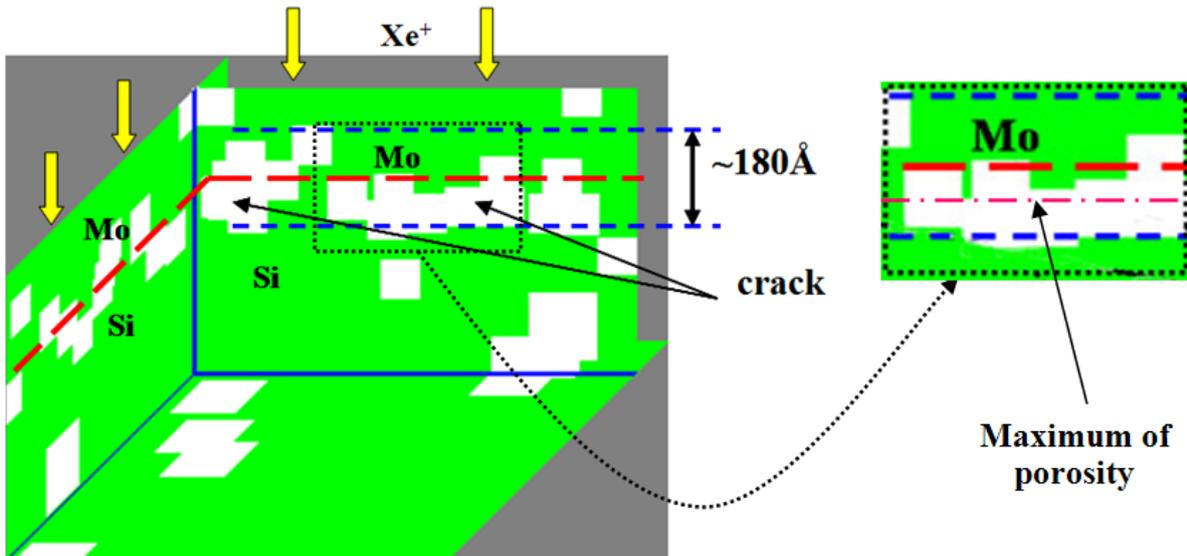
**Fig. 10** Illustration of long-size defects structure formation, which perpendicular  $Xe^{++}$  flow, in the two-layer substrate consisting of layer *Mo* (width is 94 Å) and layer of crystal *Si* (width is 543 Å) is presented. White color corresponds porosity, and green color lack of porosity in this point. Temperature is 700K,  $Xe^{++}$  ions energy is 5keV, irradiation dose is  $10^{16} \text{ cm}^{-2}$ .
