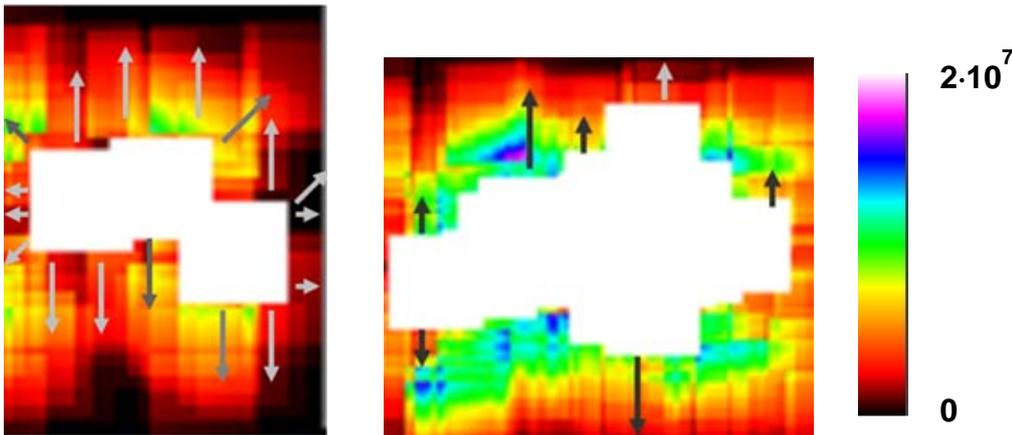
**Fig. 17** Tension gradient corresponding long-size defects structure formation for same parts of substrate sections is presented. Palette of correspondence of tension gradient value and color is presented in right part of picture. Grey arrows correspond directions of tension gradient.
