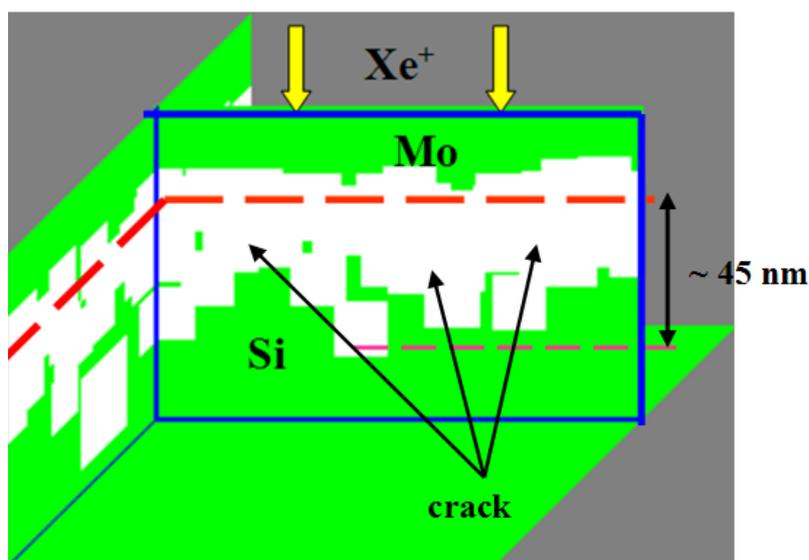
**Fig. 13** Illustration of formation of long-size structures of defects in the bilayer substrate consisting of layer *Mo* and layer of crystal *Si* is presented. *Mo* width is 94 Å, *Si* width is 543 Å. White color corresponds porosity, and green color lack of porosity in this point. Temperature is 1000K,  $Xe^{++}$  ions energy is 5keV, irradiation dose is  $10^{17}$   $cm^{-2}$ .
