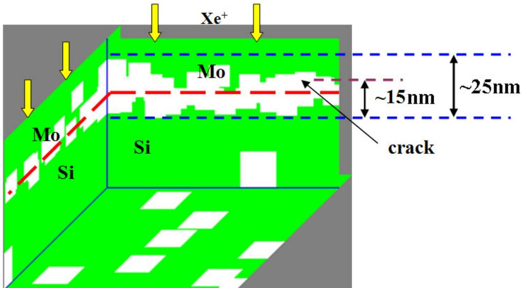
**Fig. 11** Illustration of formation of long-size structures of defects in the bilayer substrate consisting of layer *Mo* and layer of crystal *Si* is presented. *Mo* width is 94 Å, *Si* width is 543 Å. White color corresponds porosity, and green color lack of porosity in this point. Temperature is 1000K,  $Xe^{++}$  ions energy is 5keV, irradiation dose is  $10^{16} \text{ cm}^{-2}$ .
