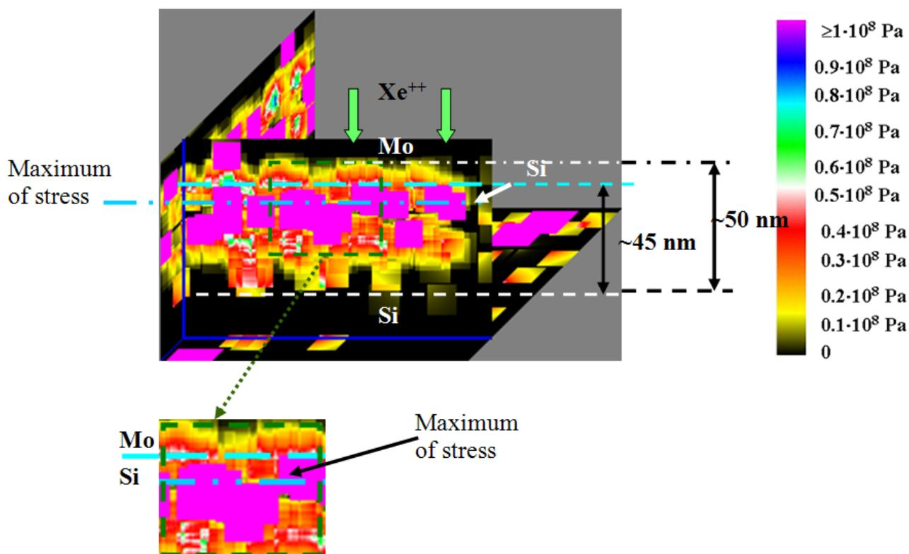
**Fig. 14** Stress corresponding with blistering in some section of substrate is presented at finish of fluctuation stage ( $10^{-4}$ s). Temperature is 700K,  $Xe^{++}$  ions energy is 5keV, irradiation dose is  $10^{16} \text{ cm}^{-2}$ . Palette of correspondence of stress value and color is presented in right part of picture.
