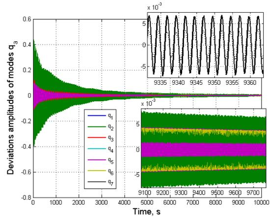
Fig. 4. Deviations of antenna modes and estimation of EKF for one of the mode (upper right)
