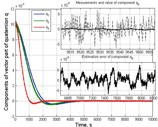
Fig. 2. Attitude quaternion of the satellite body, star tracker measurements (upper right) and estimation of EKF (lower right)
