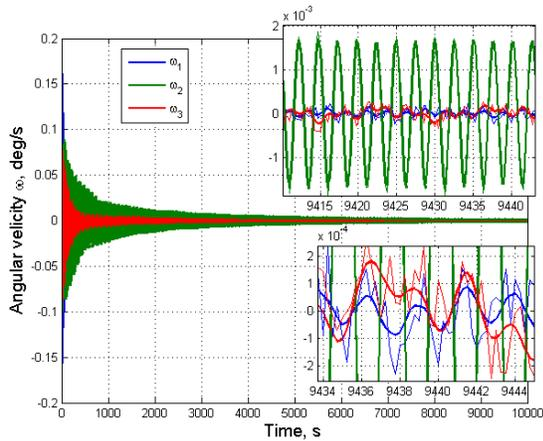
Fig. 3. Angular velocity of the satellite body, angular velocity sensor measurements (upper right) and estimation of EKF (lower right)
