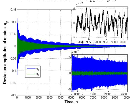
Fig. 5. Deviations of panel modes and estimation of EKF for one of the mode (upper right)
