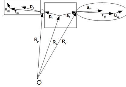
Fig. 1. Scheme of satellite with flexible elements
