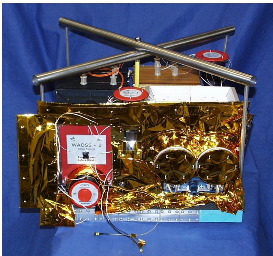
Payload platform of BIRD with assembling tools (without the hyperspectrometer)
