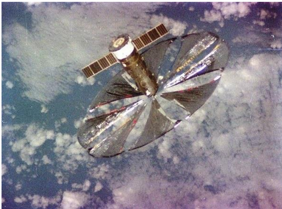
Fig. 3. A photo of the unfolded thin-film structure of the «Znamya-2» experiment from the «Mir» space station. Source: S.P. Korolev Rocket and Space Corporation "Energia".
